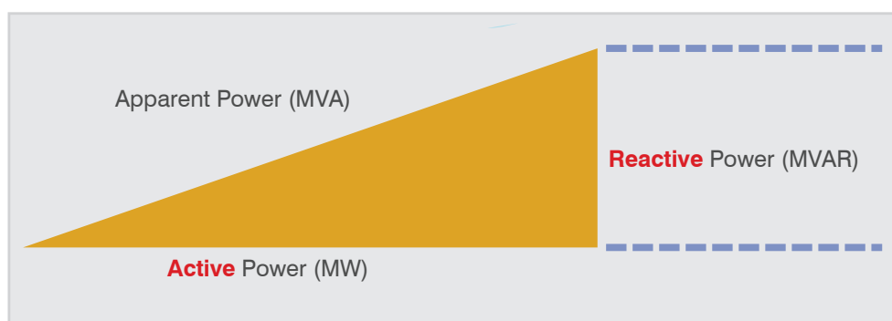
Figure 3 Active power (MW), Reactive power (MVAR) and Apparent power (MVA)
